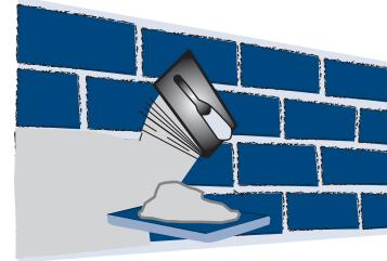
If you are applying more than one coat, you will need to let each coat dry for at least 3 - 7 days. You will then need to scour each coat with a sharp object to provide a good surface for the second coat of render to bond to.
