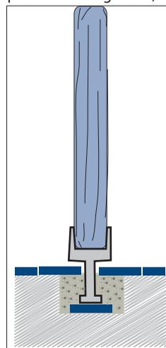
33% of the post is in the ground to achieve sufficient strength. Alternatively you can purchase a post shoe or metal stirrup which is specially designed for posts.
