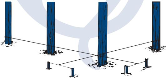
The depth will depend on the length of the post, normally one third of the post length must go into the footing, with a minimum footing depth of 230mm. The footing diameter should be three times the diameter of the post being placed.
