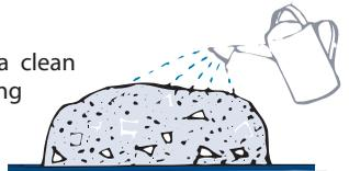
Add the coarse aggregate, mix all three ingredients thoroughly again until the colour is consistent. Finally add your measured quantity of water, sprinkle the water slowly over the mix, stopping frequently to turn over the mix until the mix is consistent in colour and texture. Do not add too much water, you do not want your mix too sloppy. Too much water means a weak concrete. The water should weigh roughly half of that of the cement added.
